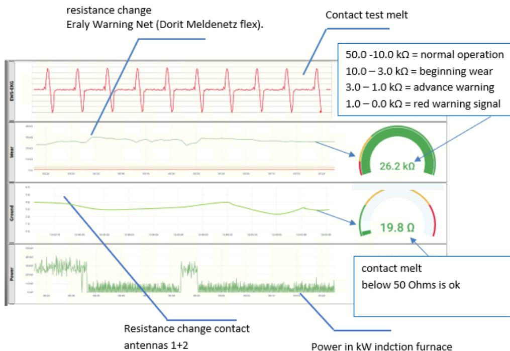
Online display of the proportional change of the refractory resistance with decreasing lining thickness
