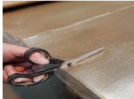
Installation of the detection mesh, instead of the mica sliding layer, easy to cut
