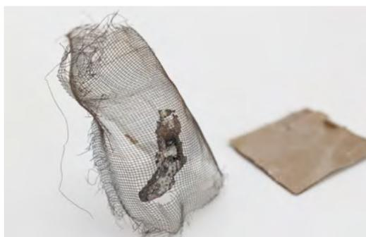
Direct melt contact with the sensor mesh
