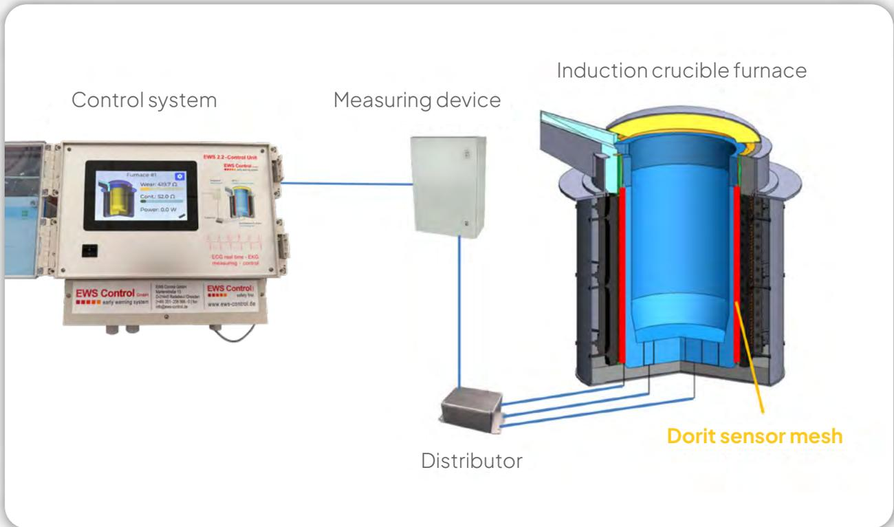
Basic structure of the Foundry Guard early warning system with monitor display, wall mounting of the control cabinet, according to customer specifications. Standard closet with clear glass door.
