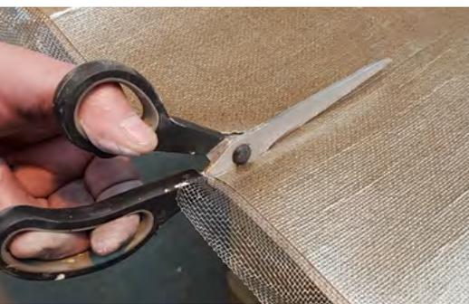
Easy adjustment of the sensor mesh
